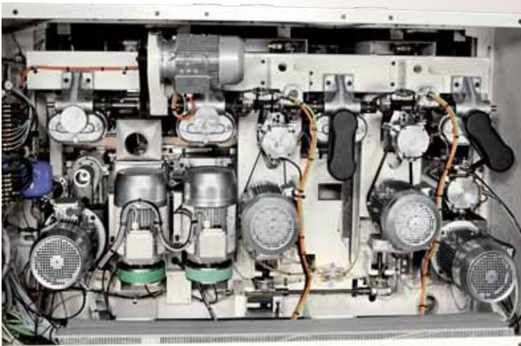
On the Superset NT each tool spindle has its own, independent motor. The machine is a truly powerful throughfeed moulder.
