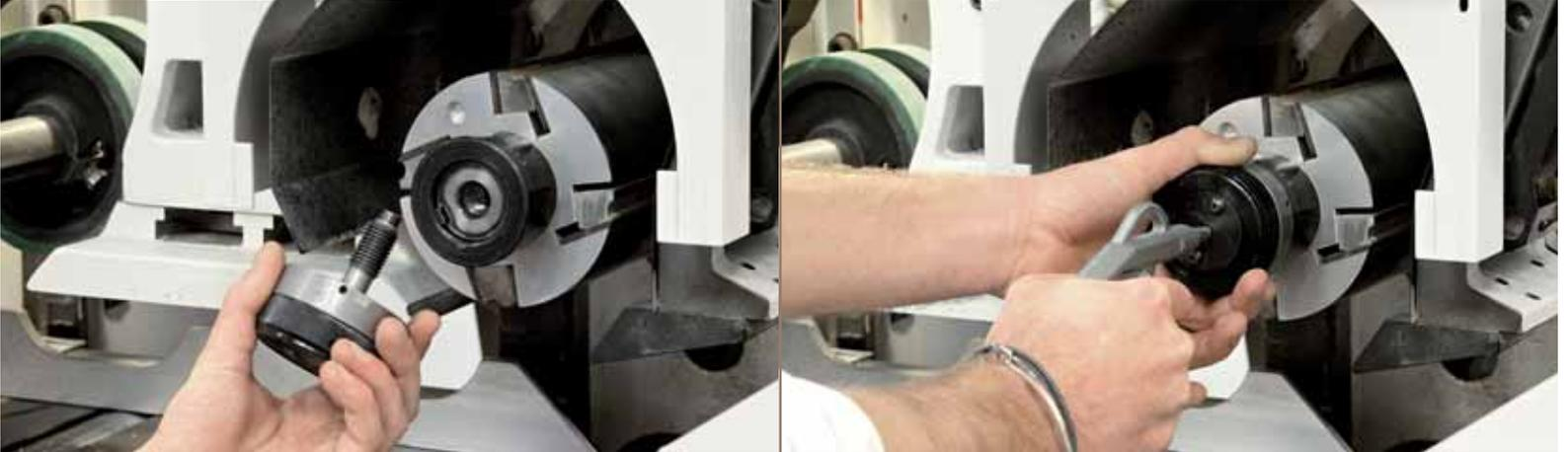
T-SET: device for tool locking/unlocking
