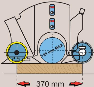
Configured for machining short parts: single workpiece feed with minimum length of 370 mm.
