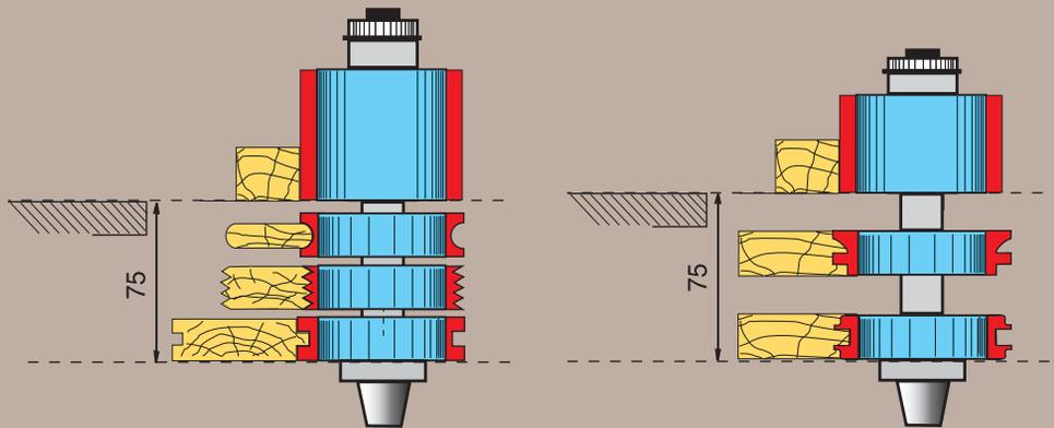
Superset NT has the innovative **SETUP/2** system fitted as standard making set-up times at part changeover up to twenty times faster.
